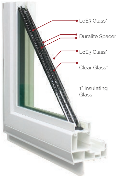
Triple Pane Glass 1" Insulated glass unit
